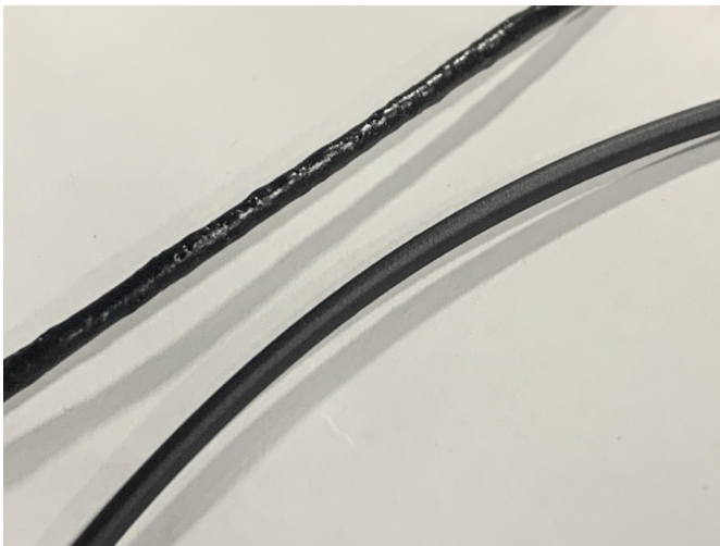
Fig. 18 The low and high-quality filaments
