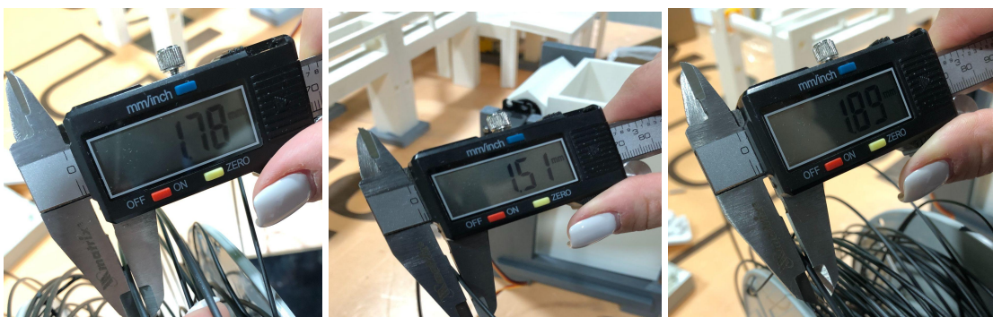
Fig. 23 Some of the results obtained during the experiment with 18 rpm screw speed
