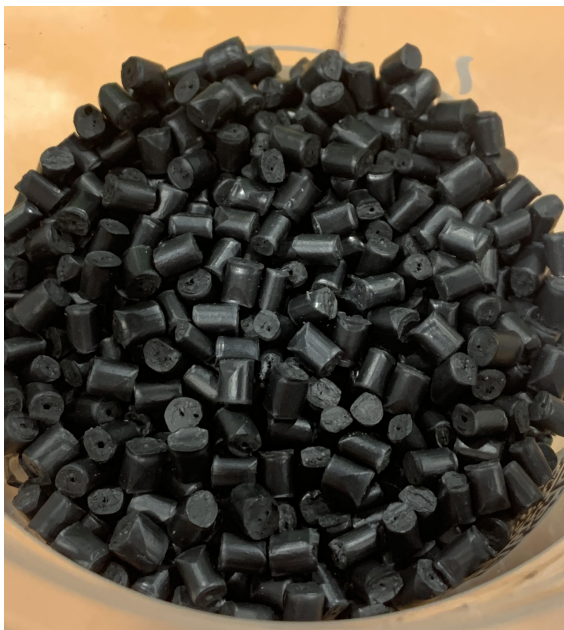
Fig. 13 Recycled ABS pellets that were used in the experiment
