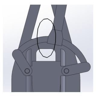
In the screenshot, you can see the path of the central part of the end rod 4. In the real model, since it is not sticked with the elastic element, it is sliding left to right, but the path remains the same. For this mechanism, also, it was quite difficult to get motion graphs that would depict the mechanism's true motion as it is also connected to an elastic link.
