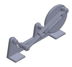
and forth. One was to make one end of the pin wider to limit its movement from one side. Another thing we implemented was to make a sleeve that would go onto the pin and stay between parts to limit the movement.
