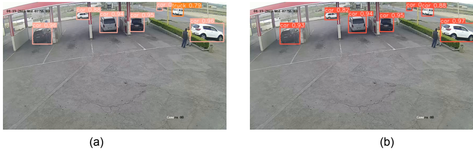
Figure 8. Object detection results of trained (a) multi-class and (b) single-class YOLOv8 models.
