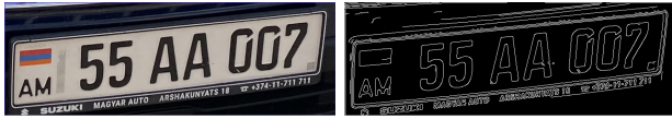
(a) Original image after cropping detected license plate. (b) Image after edge detection is applied
