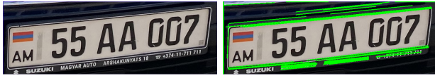
(a) Original image after cropping detected license plate (b) Image after Lines Detected using Hough Transform
