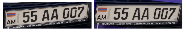
(a) Original image after cropping detected license plate (b) Image after the Orientation Correction
