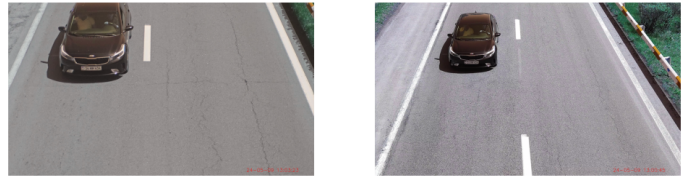
Fig. 8: Processed Result Example No Violation: Threshold 90km/h: Registered: 67.22 km/h
