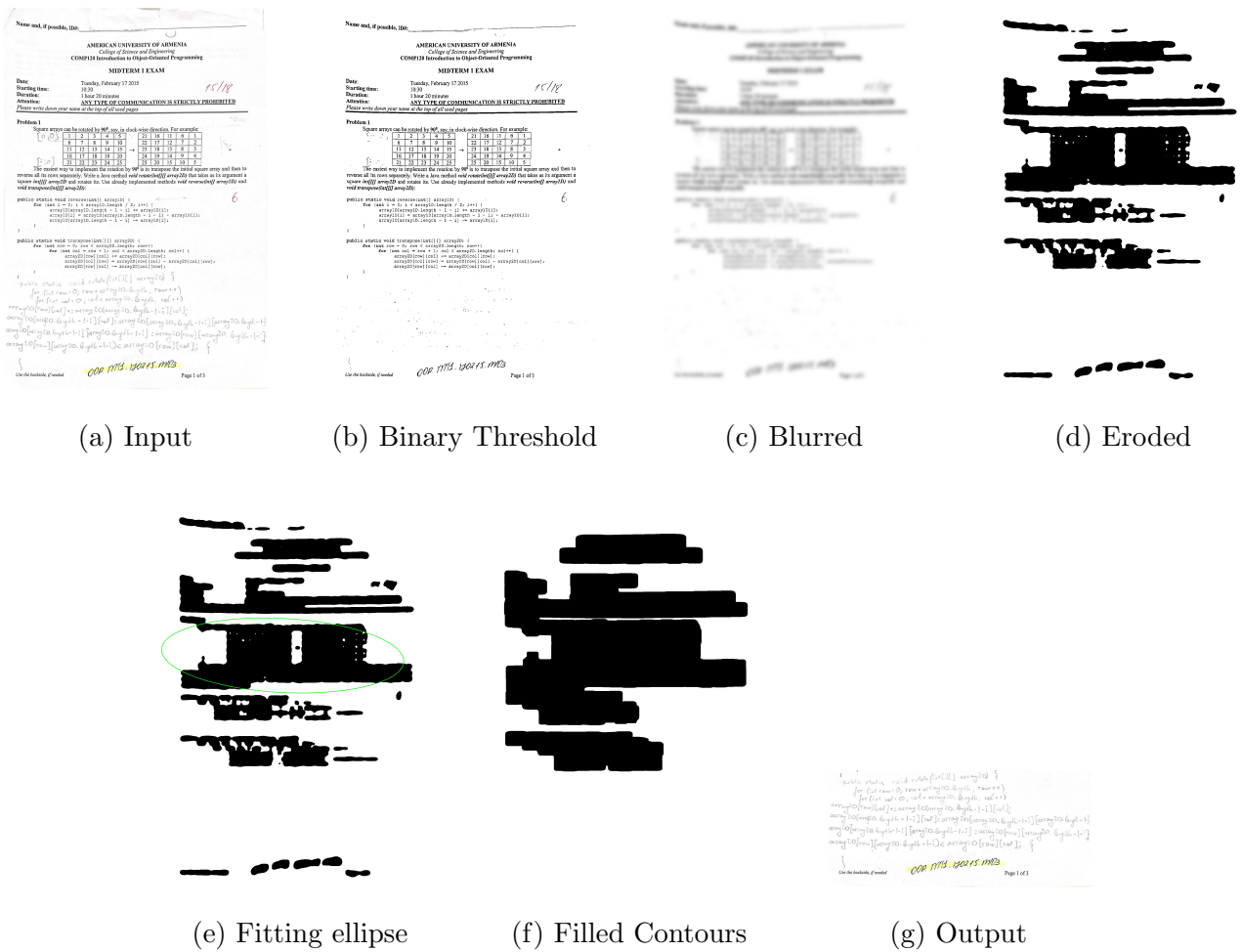
Figure 3: Handwriting Isolation by Contour Detection
