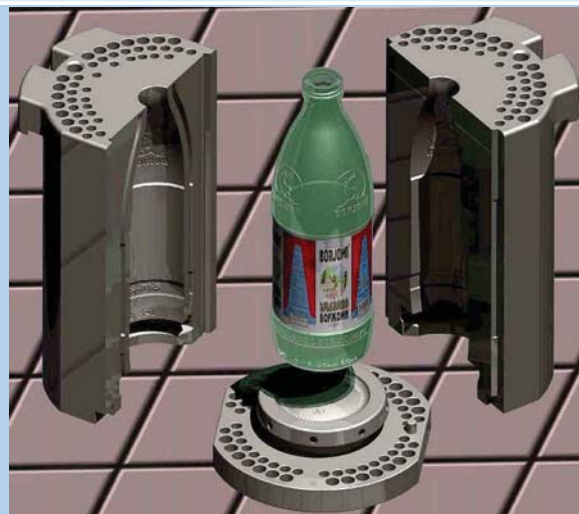
Fig. 8 Copying the bottle face and extending to split the remaining workpiece into side pieces.
